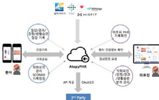
Fig. 1. System architecture of AtopyPHR
